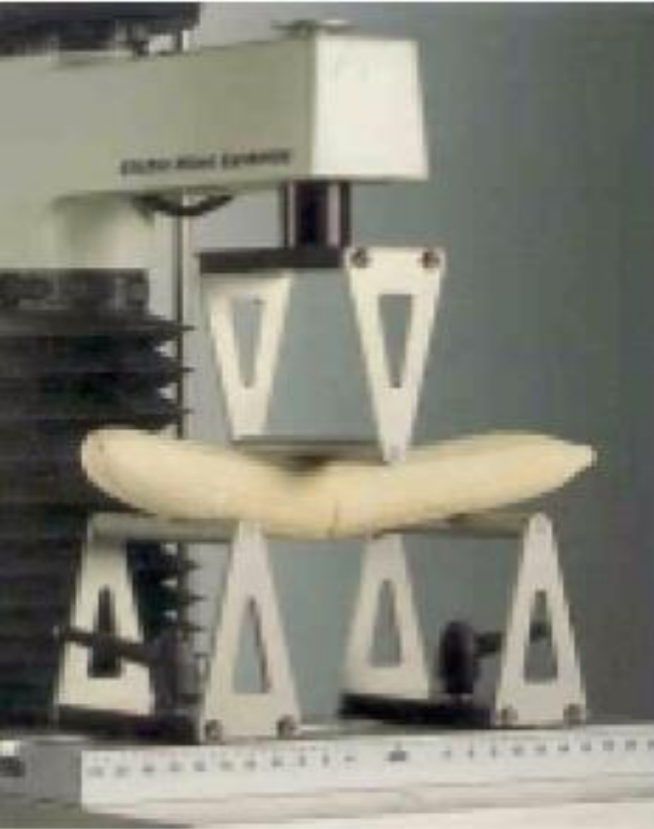
THREE POINT BEND RIG
