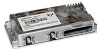
DS300 ORBCOMM satellite transceiver with on-board application processor, power conditioning circuitry, battery charger and digital/analog IO's.
