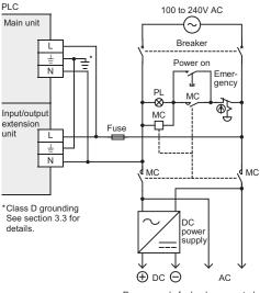
Power supply for loads connected to PLC output terminals
