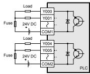
2. External Wiring of Source Output Type
